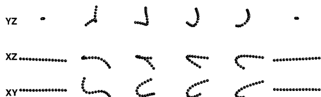
FIG. 16. U-turn (Group 3B) configurational dynamics exhibited by flexible fibers ( k^{(B)*}=50 , C^0=0.5 ) drifting toward C=\infty orbits in simple shear flow.
