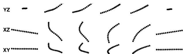
FIG. 17. Flexible spin-rotation (Group 3B) configurational dynamics exhibited by relatively stiff fibers ( k^{(B)*}=70 , C^0=0.5 ) that settle into intermediate orbits in simple shear flow.
