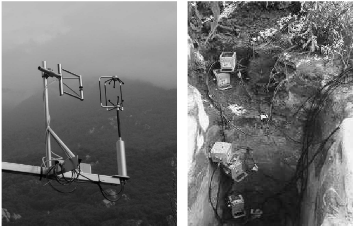
Fig. 2. Instrumentation at the site ‘Bosco di Sotto’. Left: asymmetric ultrasonic anemometer combined with a fast-response krypton hygrometer. Right: soil moisture detection by TDR-probes.
