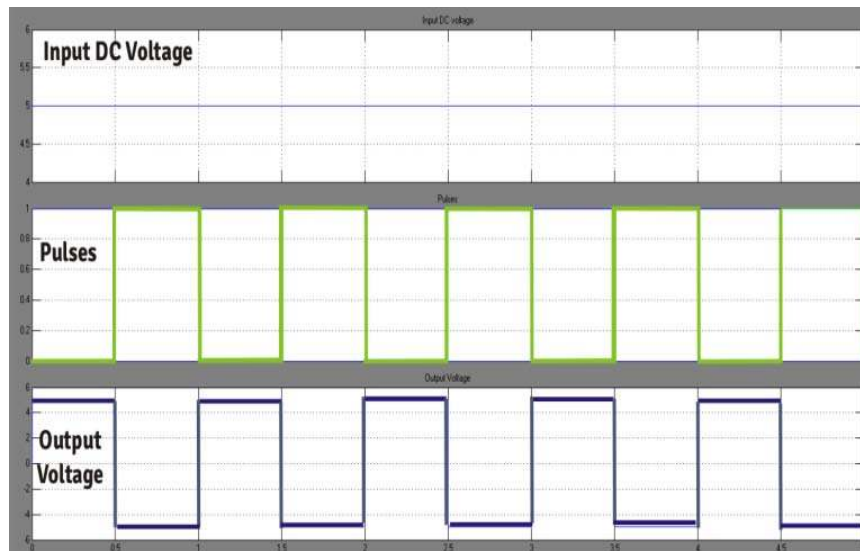
Figure 12: Simulated results of Gating Pulses and input and output voltage.
