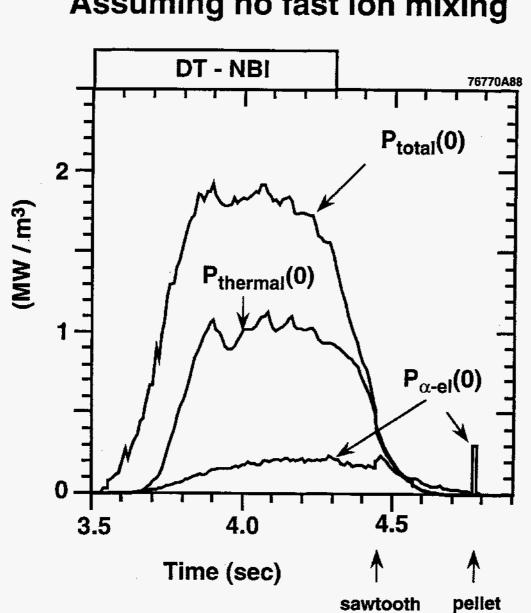
Central Fusion Power Assuming no fast ion mixing
