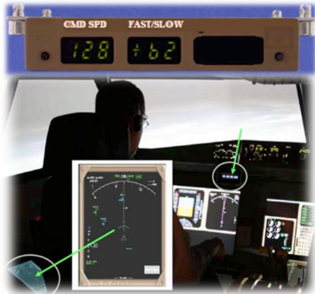
Figure 3. Example ASTAR Electronic Flight Bag (EFB) implementation with ADS-B Guidance Display (AGD).
