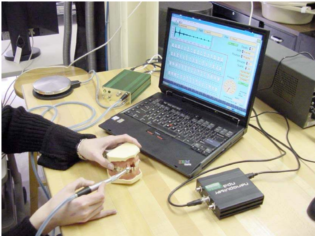
Fig. (2). Picture of the latest generation of the ultrasonographic periodontal probe system.
