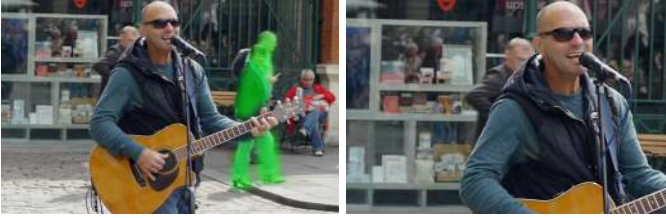
Fig. 15. Our system cannot produce good results in the case where the distraction overlaps with the main object. (left) Original videos. (Right) Our results. The distracting object is marked in green. The guitar and the distracting pedestrian overlap for several frames, causing part of the guitar to be removed by our method.
