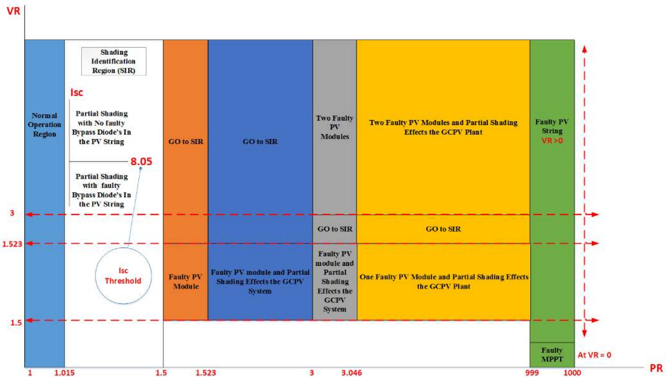
Fig. 8 PR vs. VR based on the analysis of the proposed PV fault detection algorithm
