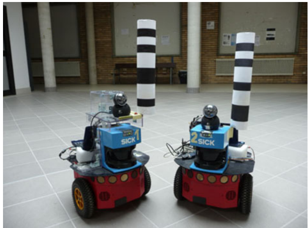
Fig. 10 Robots P3-DX used for real tests. A bar code marker is used to distinguish the robots
