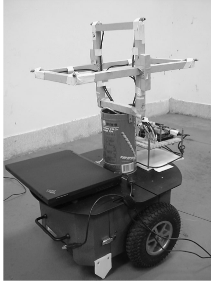
Figure 2. Digital microphone array mounted on the robot.
