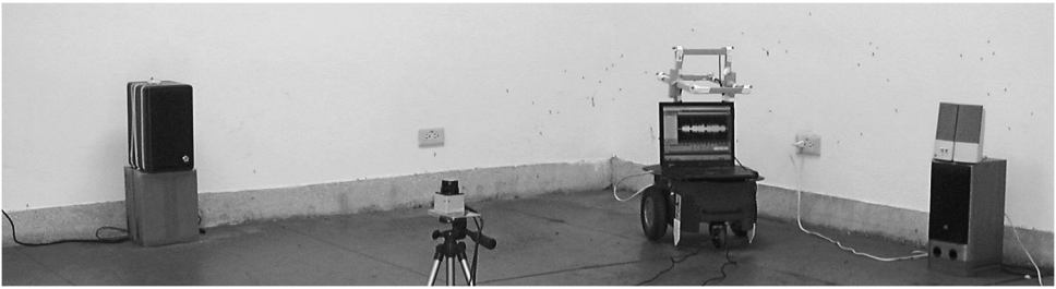
Figure 7. Spatial relation of the speaker, robot and laser range finder for C2.
