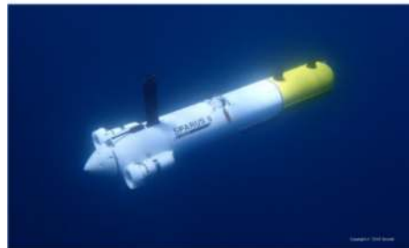
Fig. 1: SPARUS-II, a torpedo-shaped AUV.
