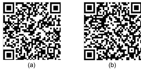
Fig. 11 Recording patterns. (a) Pattern for even-numbered layer. (b) Pattern for odd-numbered layer.
