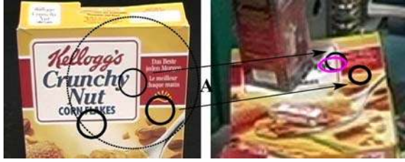
Figure 6. Left: a candidate ( thin ) and 2 of 20 supports within the large circular area. Right: the candidate is propagated to the test image using the affine transformation A of the support on the right ( thick ). Refinement adapts the shape to the perspective effects ( brighter ). The other support is mismatched to a region not visible in this close-up.
