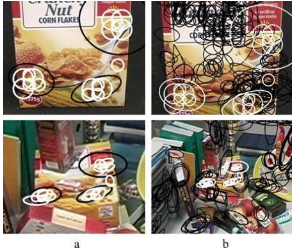
Figure 4. (a) Early propagation generates 17 correct matches (bright) out of 113. These are located around the initial 3 correct matches (dark). (b) The configuration after early expansion has 20 correct matches (bright) and 310 mismatches (dark).
