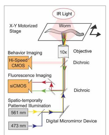
FIGURE 1 | Schematic of the illumination and imaging systems.
