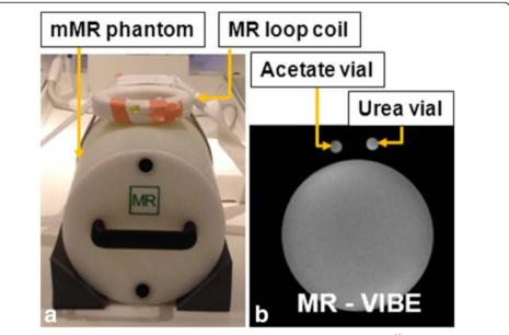
**Fig. 2** mMR water phantom setup. **a** Photo of setup with mMR water phantom. The <sup>13</sup>C loop coil is marked with arrows. **b** <sup>1</sup>H-MRI with urea and acetate vials marked with arrows
