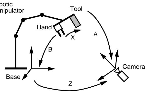
Fig. 2. Robot/eye ( $\mathbf{Z}$ ) and hand/tool ( $\mathbf{X}$ ) calibration. The tool is mounted onto the gripper and tool motions are determined by observing tool feature points with a camera. The world frame is, in this case, identical with the camera frame.
