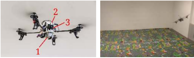
(a) A closeup of our quadrotor: 1) down-looking camera, 2) Odroid with an OptiTrack motion-capture U3 quad-core computer, 3) PIX-HAWK autopilot. (b) Our flying arena equipped with an OptiTrack motion-capture system (for ground-truth recording).
