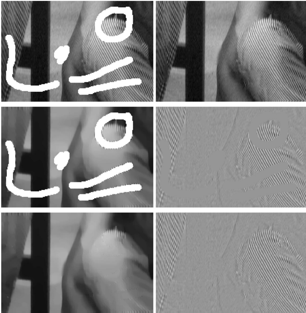
Fig. 2. Basic algorithm proposed in this paper. The original image in the first row, left (a section of Fig. 1) is decomposed into a structure image and a texture image, [31], second row. Note how the image on the left mainly contains the underlying image structure while the image on the right mainly contains the texture. These two images are reconstructed via inpainting, [5], and texture synthesis, [10], respectively, third row. The image on the left managed to reconstruct the structure (see for example the chair vertical leg), while the image on the right managed to reconstruct the basic texture. The resulting two images are added to obtain the reconstructed result, first row right, where both structure and texture are recovered.
