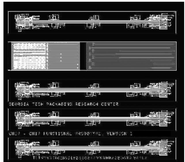
Figure 6: Top View of the Completed SOP SSN Test Vehicle Design in Cadence APD
