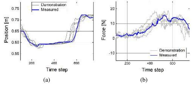
Fig. 10: The measured (a) position profiles and (b) force profiles of robot endpoint in  $y$  direction during task reproduction.
