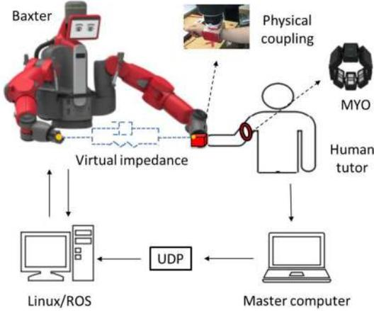
Fig. 4: The experimental setup for skill demonstration
