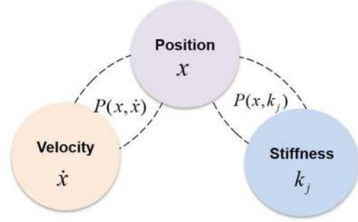
Fig. 2: Graphical representation of the two joint Gaussian distributions  $\mathcal{P}(x, \dot{x})$  and  $\mathcal{P}(x, k_j)$ , respectively, encoded in each of two continuous HSMMs of  $K$  states. The output distribution of each state of these two HSMMs is represented by a Gaussian locally encoding variation and correlation information between position and velocity, and position and stiffness, respectively.
