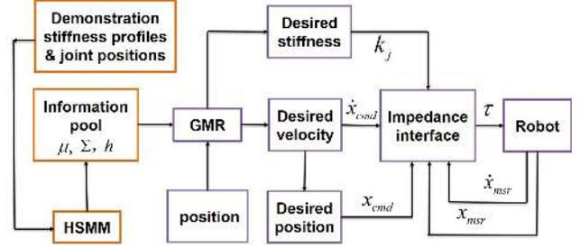
Fig. 3: The control diagram during the reproduction phase.
