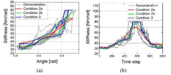
Fig. 7: The demonstrated and learned stiffness profiles of joint S1 with respect to (a) joint angle and (b) time step.
