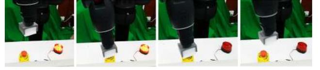
Fig. 5: Successful task reproduction of the button-pressing task. From left to right: the starting pose, moving to the button, pressing the button and finally leaving the button.
