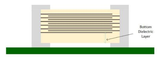
Figure 6. Thicker Bottom Dielectric Capacitor.
