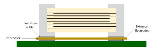
Figure 5. Interposer Capacitor.
