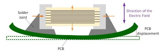
Figure 2. The mechanism for singing capacitor phenomenon.
