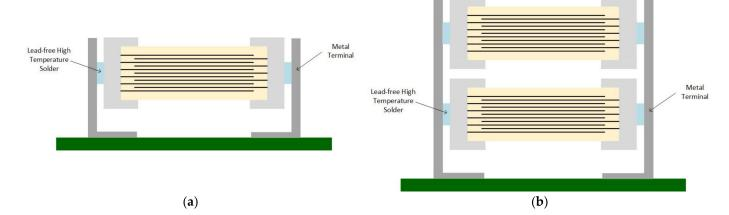
Figure 4. Metal terminal capacitors (a) Single MLCC type; (b) Dual MLCC Type.
