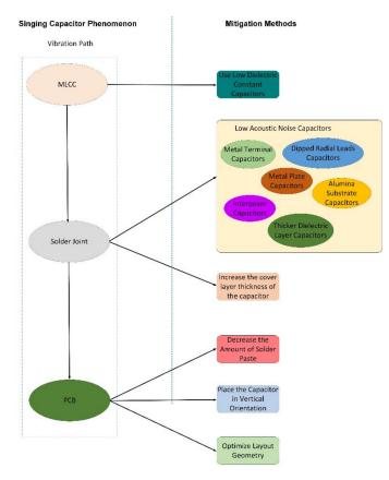
Figure 3. Solutions for singing capacitor phenomenon.
