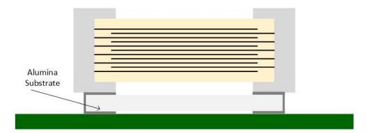
Figure 7. Alumin Substrate Capacitor.
