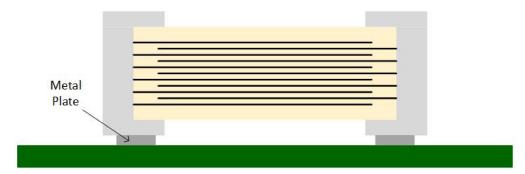
Figure 8. Metal Plate Capacitor.
