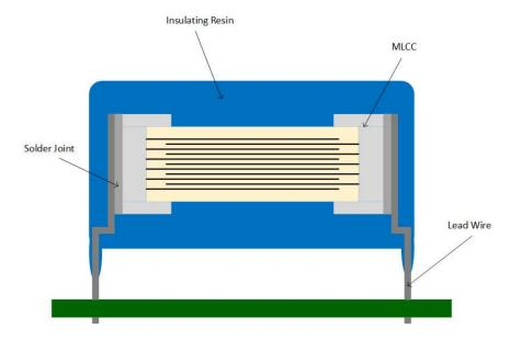
leads capacitors and the fact that they are through-hole capacitors makes them unsuitable for designs with dimensions restrictions.
