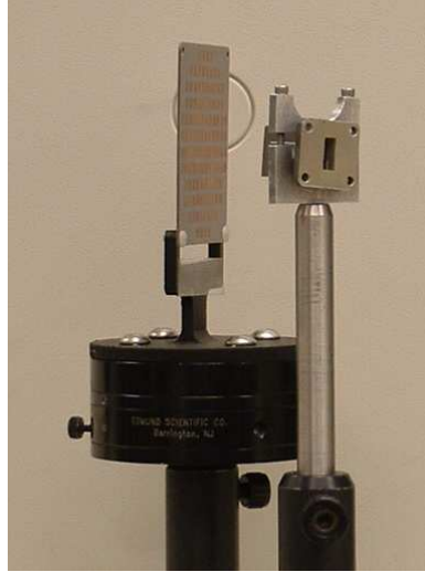
Figure A.8: The lens was fed by a 10-dB gain horn antenna. Scanning was simulated by rotating the lens relative to the feed-horn.
