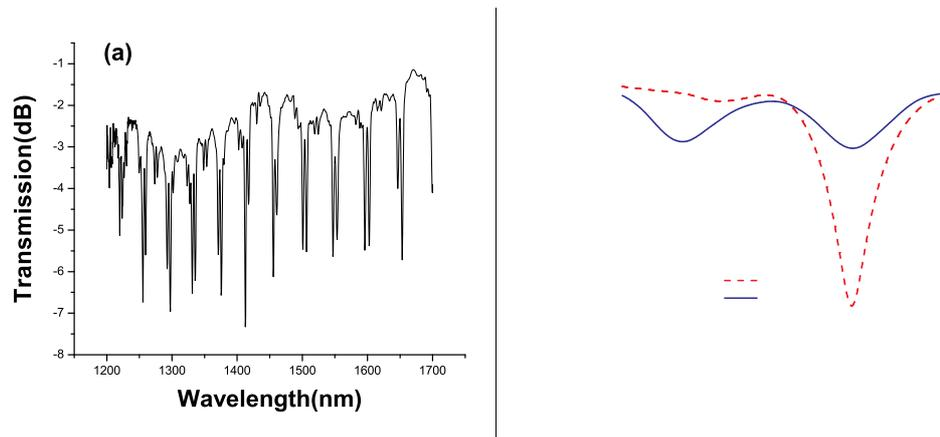
Figure.2 PDL of the used 45°-TFG measured by the EXFO PDL characterization tool kit
