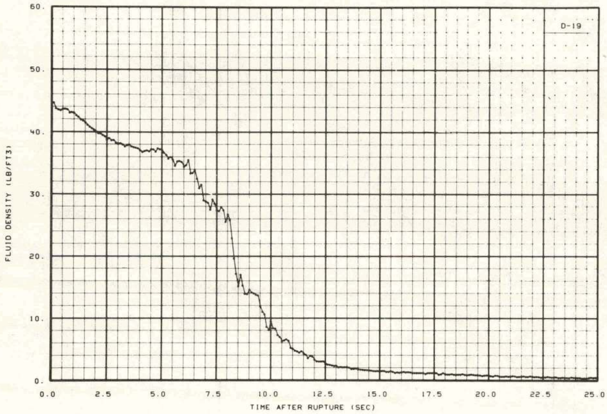
Fig. A-25 Pump outlet fluid density -- Test 1010.
