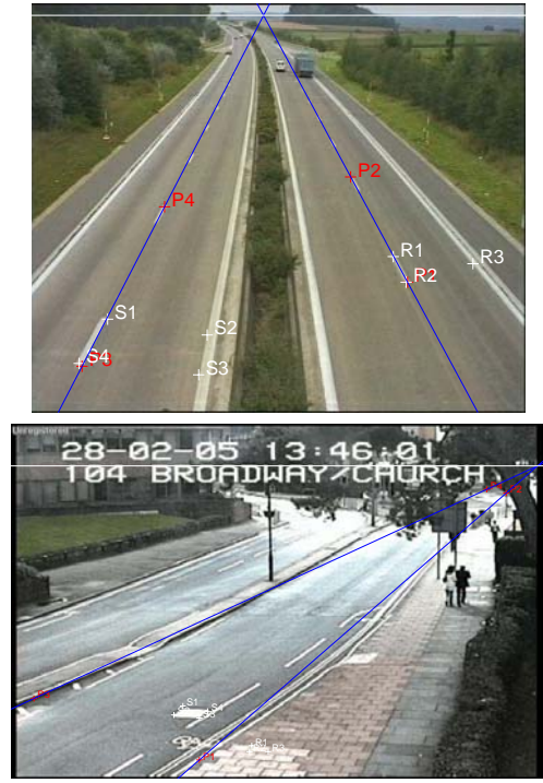
Figure 2: Example of vanishing line construction. The blue lines represent pairs of parallel lines intersecting on the vanishing points. The white line represents the vanishing line. \{S1, \dots, S4\} and \{R1, \dots, R3\} are used for known angles and length ratio selection
