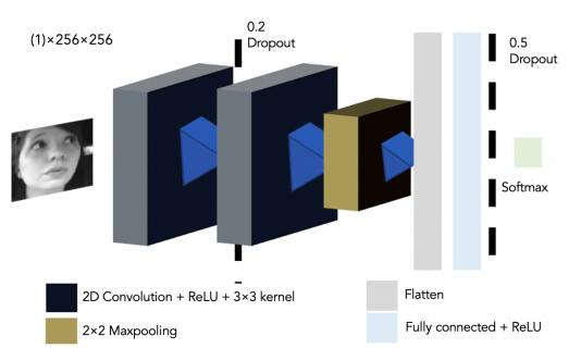
**Figure 2.** Two-dimensional CNN Network Architecture used to predict the six different proposed standard driving gaze areas with a one-channel (1) image input.
