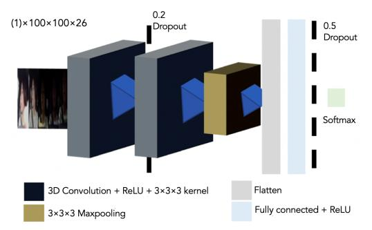
**Figure 3.** Three-dimensional CNN architecture used to predict the six different proposed standard driving gaze areas with a one-channel (1) sequence of frames input.
