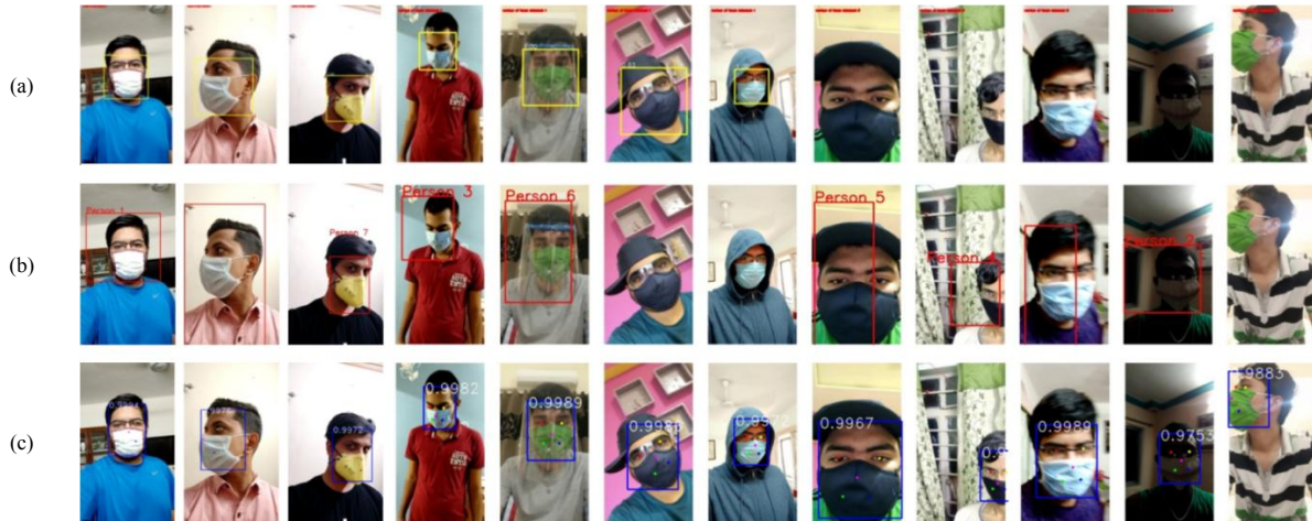
Fig. 5. Detection results of different algorithms on the dataset video frames. (a) YOLO-face. (b) YOLOv3. (c) RetinaFace.
