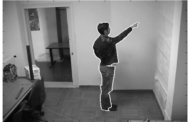
Figure 2: Silhouette detected by the GVF snake in a frame acquired in the side camera setup.
