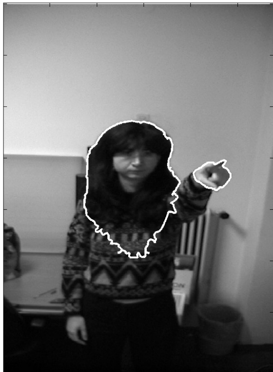
Figure 3: Pointing hand and head detected by the GVF snake in a frame acquired in the frontal camera setup.
