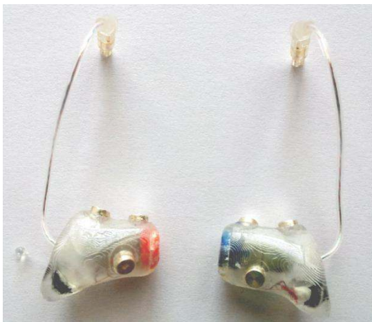
Figure S3: Exemplary in-Ear-EEG devices. Each device has three EEG electrodes attached (© 2016 IEEE. Reprinted, with permission, from Fiedler L, Obleser J, Lunner T and Graversen C 2016 Ear-EEG allows extraction of neural responses in challenging listening scenarios – a future technology for hearing aids? Eng. Med. Biol. Soc. (EMBC), 38th Annu. Int. Conf. IEEE, 38 5697–700). To create the in-Ear EEG devices, a trained audiologist took impressions of the ear canals, which were used to print 3D shells of each individual ear canal. Three holes were drilled in the shells to insert the electrodes, which were connected by short wires to a standard 3-pin Hi-PRO EASYFIT plug. Electrodes were made from a fine silverthread with a diameter of 3,00 mm cut into slices of 2,00 mm (Ravstedhus, Denmark).
