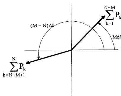
Fig. 5. Graphic representation for the vectoric sum of the two phasors of Eq. (5).
