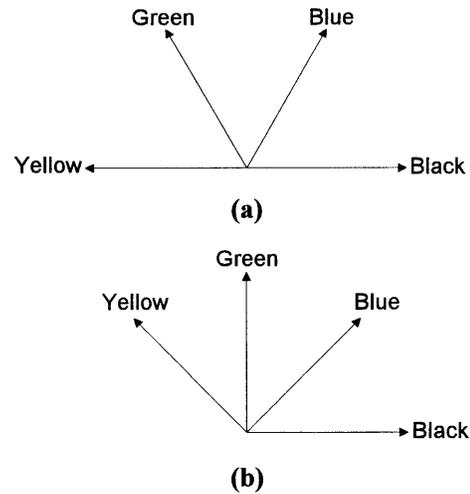
Fig. 3. Possible color-phase codes for four-color images for (a) a 180° phase range and (b) a 135° phase range (the optimal phase range).
