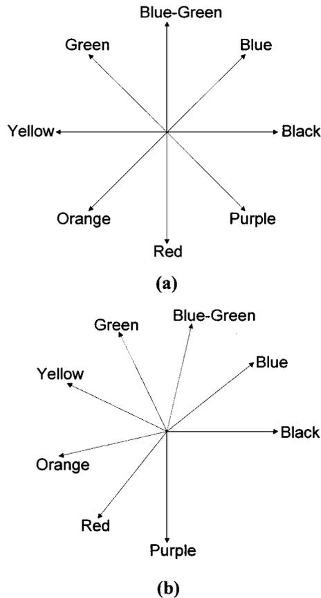
Fig. 2. Possible color-phase codes for eight-color images for (a) a 315° phase range and (b) a 270° phase range.
