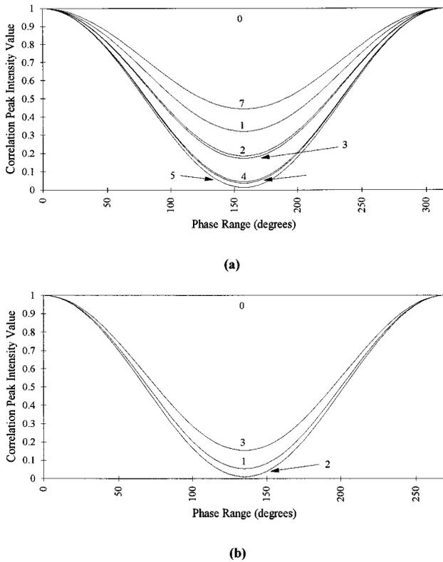
Fig. 8. Computer-simulation results for the correlation center intensity values versus the phase range for different color-code rotation steps. The numbers near each curve indicate the rotation steps. (a) An eight-color scene and (b) a four-color scene.
