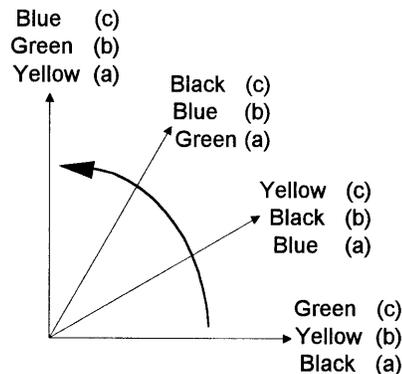
Fig. 4. Image color-code rotation: (a) the original color-phase code, and color transformations for (b) a one-step and (c) a two-step counterclockwise rotation.
