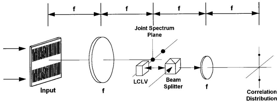
Fig. 6. Schematic diagram of the setup for a real-time JTC.
