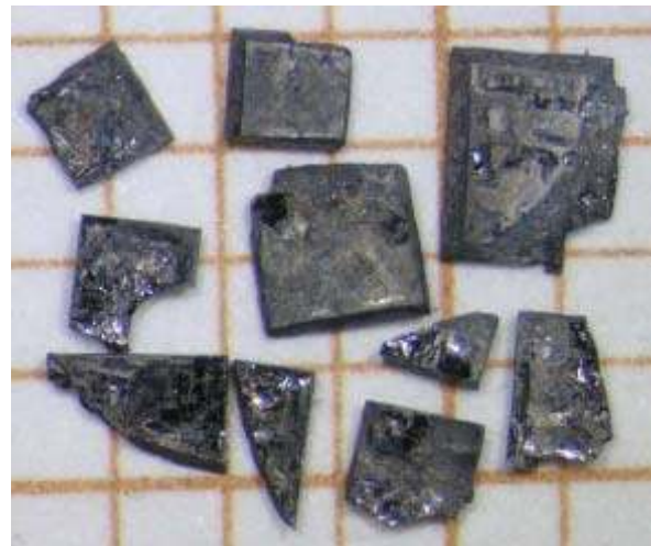
Fig. 4. Single crystals of \text{Ba}_{0.9}\text{Rb}_{0.1}\text{Fe}_2\text{As}_2 on a millimeter grid.
