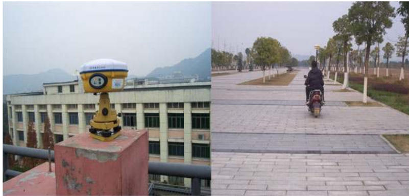
Figure 4. Setup of base and rover stations.
