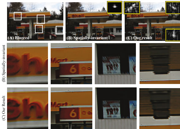
Fig. 6. Deblurring result. (A) Blurred image, (B) Deblurred image using spatially invariant approach, (C) Deblurred result using our system. Recovered blur kernels at few locations are shown in yellow boxes.
