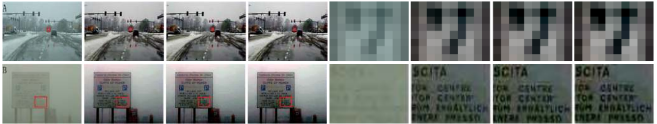
FIGURE 5. From left to right: the original images A and B, and the defogged images obtained by MSRCR, multi-channel convolution operation, secondary guided filter, the local amplification effect of the red box of the original images, the local amplification effect of the red box of the defogged images are obtained by MSRCR, multi-channel convolution, and secondary guided filter.
