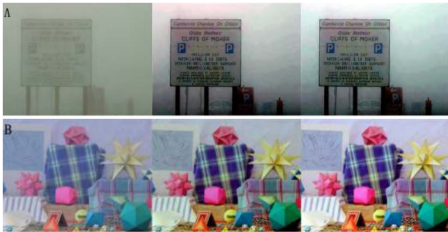
FIGURE 6. From left to right: the original images A and B, and the defogged images are obtained by secondary guided filter, white balance operation.
