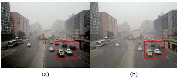
FIGURE 9. Difference in deconvolution methods indicating dehazing result using (a) Lucy-Richardson and (b) alternating direction methods of multipliers
