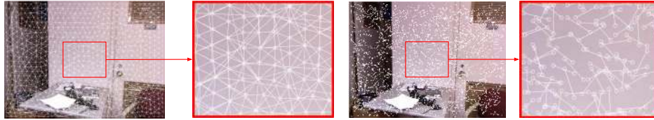
Figure 9: Point pairs generated through superpixel segmentation [14] (left) versus point pairs generated through random sampling with distance constraints (right).
