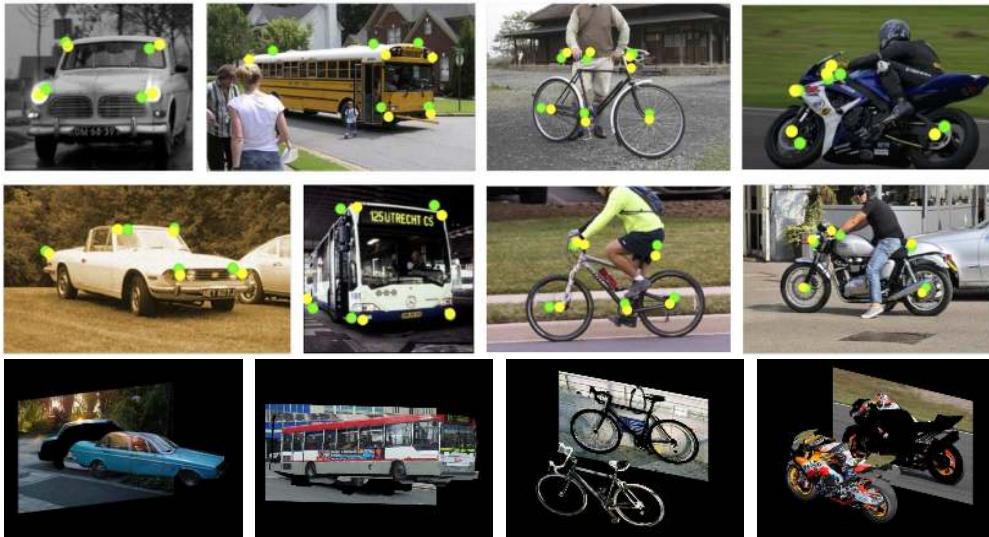
Figure 7: Examples of landmark localization results from different categories of PASCAL3D are shown in the first two rows. Visible 3D landmarks are projected back to the image. The yellow dots are groundtruth locations and the green dots are the estimation. The last row shows example pop-up results of different object classes.
