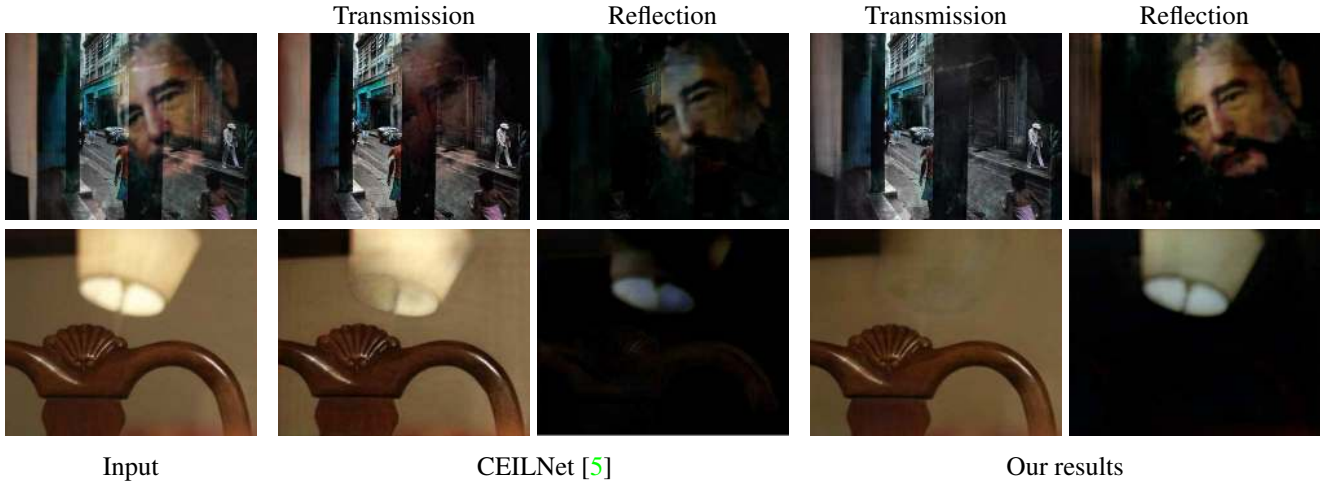
Figure 1: Results by CEILNet [5] and our approach on real-world images. The top row shows a real image from the CEILNet dataset with a window reflecting a poster of a human face; the bottom row shows an image taken by ourselves, with a lamp as the reflection. From left to right: the input images, CEILNet results and our results. Note that our approach trained to learn both low-level and high-level image statistics successfully removes the reflection layers of the face and lamp, while CEILNet does not.
