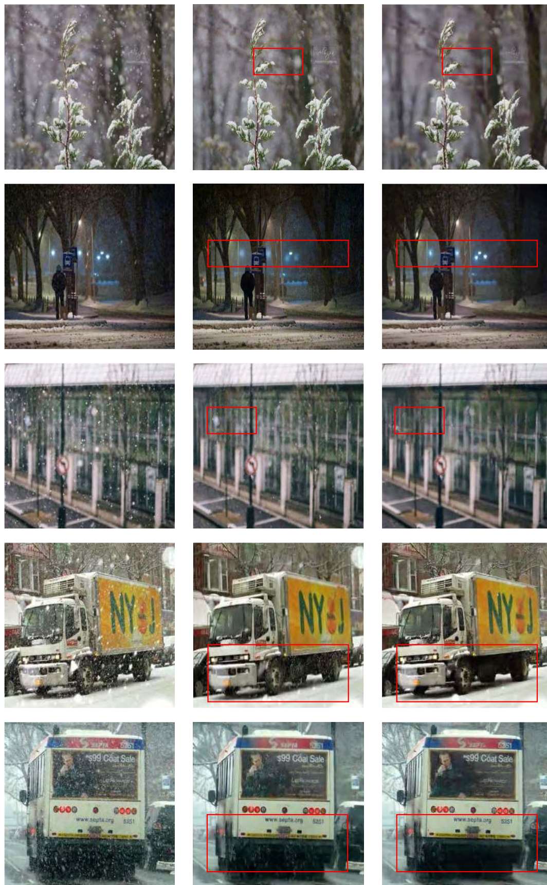
FIGURE 10. Real world snowy images and results from state-of-the-art methods. From left to right: Input real world snowy images, results of DesnowNet, results of our method.
