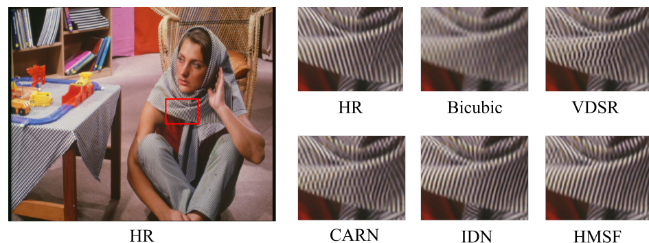
Figure 17. Failure case. A failure example of 2\times SR; our HMSF cannot correctly restore the direction of the stripe of the textile, with its complex detail and misleading information.
