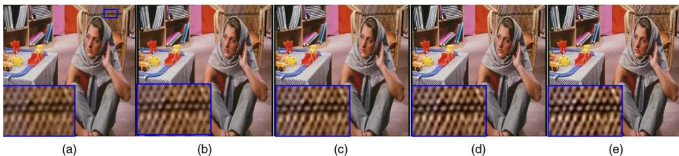
Fig. 11 The SR results (before back-projection) obtained by different Gaussian deviations: (a) 0.45, (b) 0.5, (c) 0.55, (d) 0.6, and (e) 0.65.
