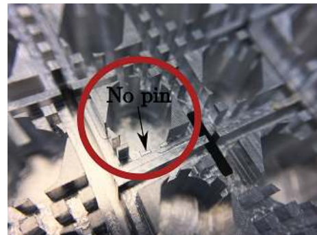
Fig. 15: Detail of the sector where a nail was incorrectly milled out.
