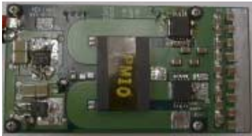
Fig. 16. 48V VRM prototype using single magnetic push-pull forward converter.
