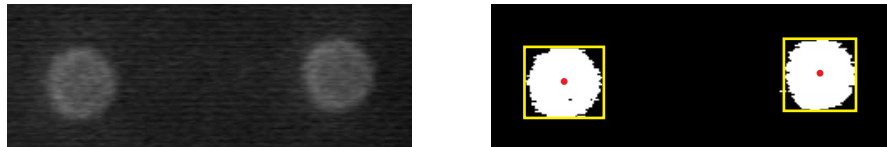
Figure 6.6: Blob analysis. The left image is a raw video frame (the actin filament is invisible due to photobleaching of the fluorophores). The right image is the result of thresholding and selecting for objects larger than 300 pixels. The calculated object centers and bounding boxes are indicated.
