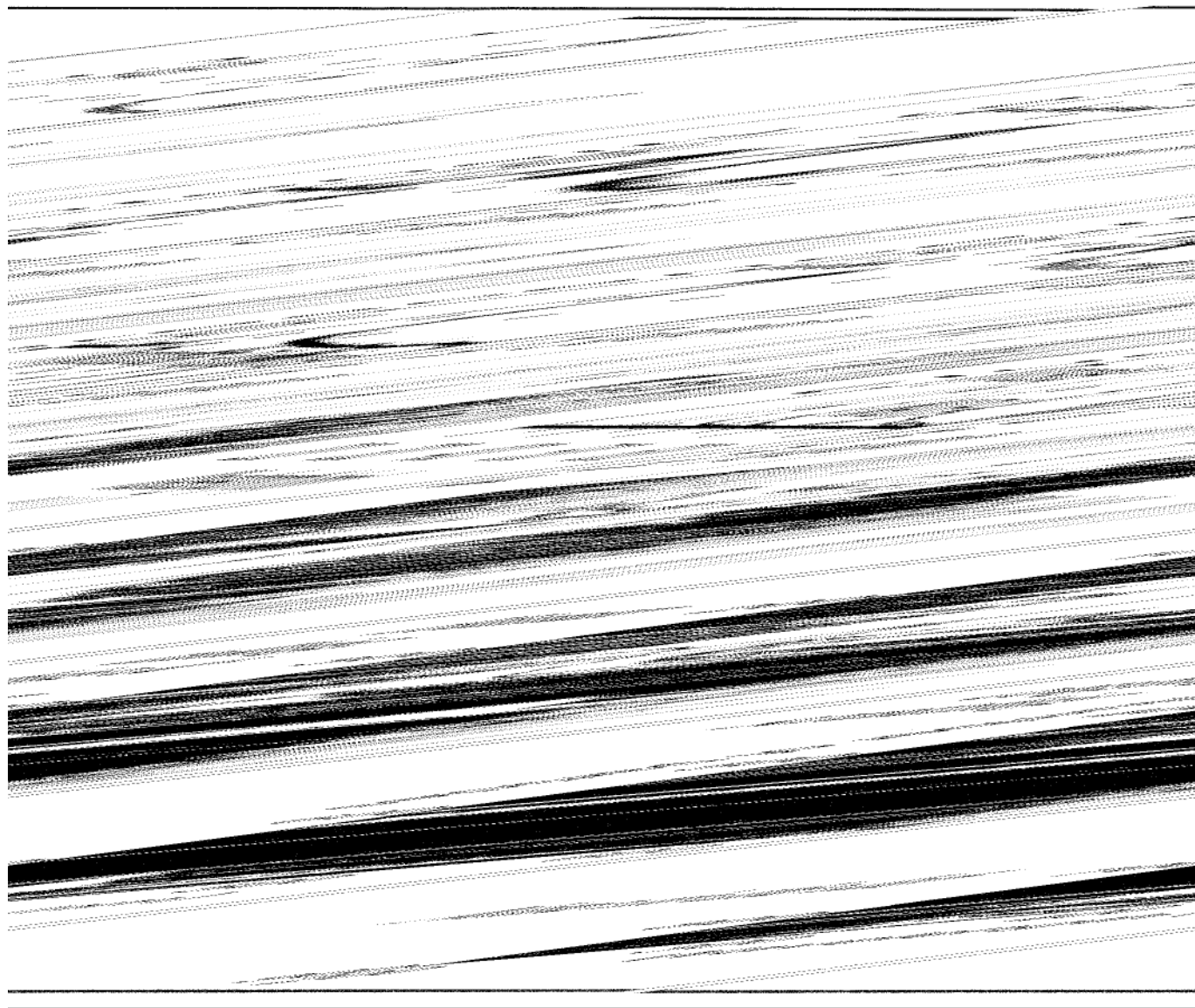
Figure 4. A display of 900 consecutive single-shot fluorescence spectra from ambient laboratory aerosols measured initially while people were talking, coughing, and scratching near the FPS inlet, and then, beginning about trace 550, when no people were in the laboratory. Typical spectral lineshapes are shown in the inset, along with the spectra from four of the primary fluorophors in biological aerosols for comparison.
