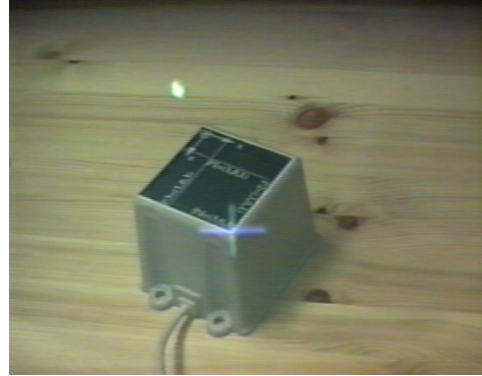
Figure 4. The calibration procedure requires the user to align a cursor as shown here with a fixed point in the world.
