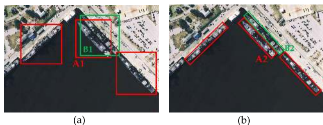
FIGURE 1. Comparison of horizontal bounding boxes and rotated bounding boxes. (a) Slender targets are detected using horizontal bounding boxes. For two adjacent ships, the horizontal bounding boxes, A1 and B1, have a large overlap area, and the box with a lower confidence score will be suppressed during the NMS procedure. (b) The oriented bounding boxes A2 and B2 wrap targets more tightly.
