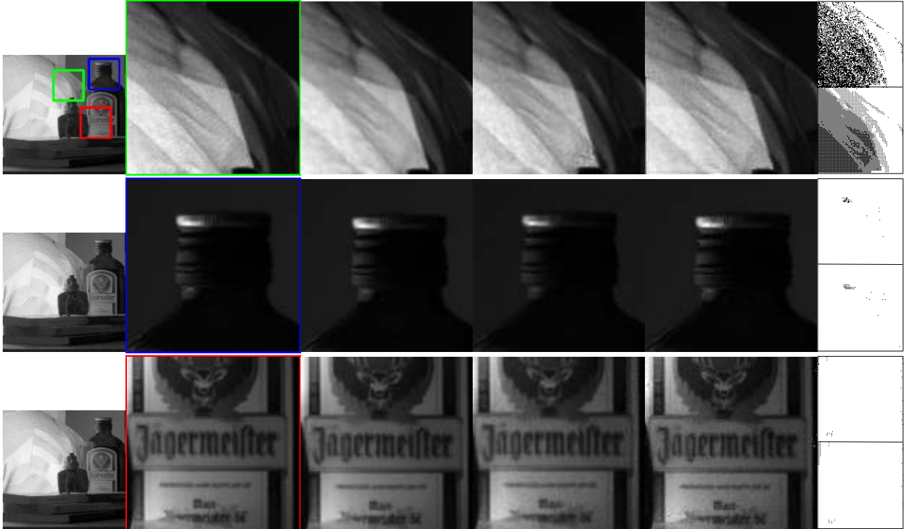
Figure 3: Synthetic data. First column (top to bottom): Ground-truth with indicated extracts, full image result obtained by the proposed approach, full image result by Schöberl et al. [15] Second to fifth column (left to right): Extracts of the ground-truth, result by the proposed approach, Schöberl et al. [15], Nayar and Mitsunaga [12]. Sixth column: Random (top) and regular (bottom) mask for each extract. Black represents unknown and white known pixels. The percentage of unknown pixels for the first extract is 65% (it is nearly the same for both the regular and non-regular pattern). For the other two extract most pixels are known (99%) so that the proposed method mostly performs denoising in these extracts.
