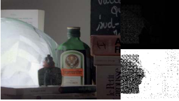
Figure 1: Example of the acquisition of an HDR scene using spatially varying pixel exposures. Left: Tone mapped HDR scene restored from the raw image. Right top: Raw image with spatially varying exposure levels. Right bottom: Mask of correctly exposed pixels (white) and under or over exposed pixels (black).
