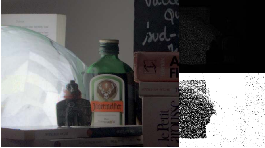
Figure 7: Real data. Left: Tone mapped HDR image obtained by the proposed approach (13.4 stops). Right top: Raw image with spatially varying exposure levels. Right bottom: Mask of unknown (black) and known (white) pixels. In the lamp area 70% percent of the pixels are unknown.
