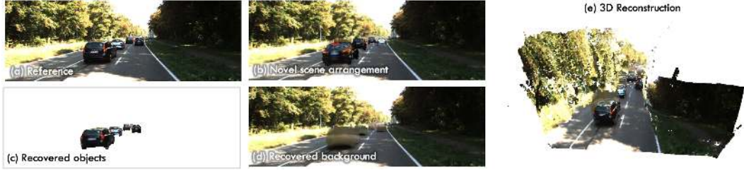
Figure 6: Scene reconstruction using our pipeline on KITTI. Our pipeline decomposes the scene into objects (c) and background (d) and recovers full geometries and appearances (e). This allows for scene manipulation, view synthesis and novel scene arrangements (b). Despite being trained on synthetic data, our pipeline generalizes well to real images without any adaptation.
