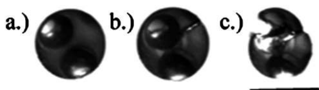
Fig. 9 Wax-stabilized double emulsion (a) before applying pressure between two glass slides and (b and c) with increasing pressure from b to c to break the double emulsion. The scale bar represents 400 \mu\text{m} .
